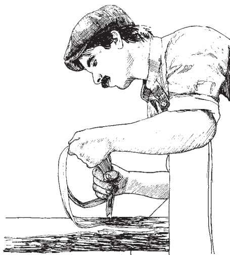
Shave off the rough outer bark of the hickory, then pull up strips of the inner bark.
