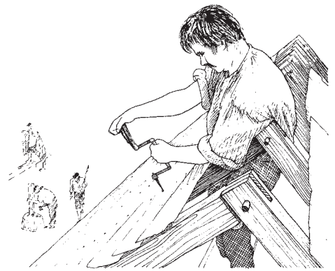
The bridle joint at the peak of the rafters is an open mortise and tenon.
