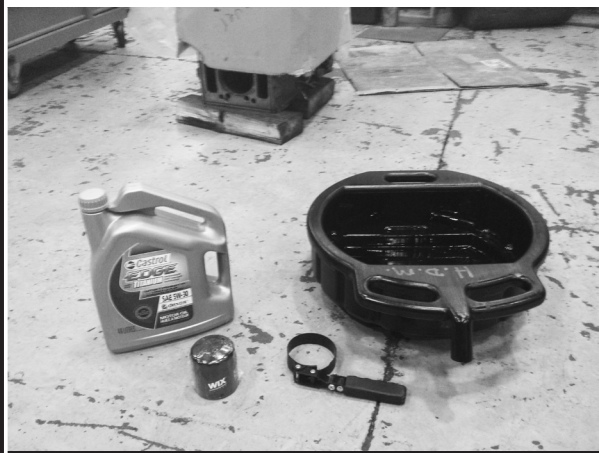
Fig 1. Oil, filter, filter wrench, oil drain pan
