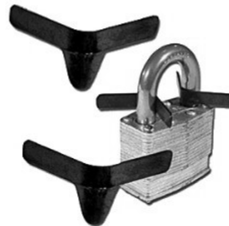
#2b: How Shims Work Inside a Padlock
