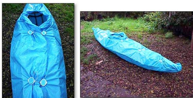
A blue tarp, 12' by 9', was used to cover the frame. You could cover your frame with animal skins if you have them. The tarp was gathered along the top of the boat and fastened together with six Grip Clips. [www.gripclips.com](http://www.gripclips.com) You can also use the rock and cord technique where you place a 1.5" rock under the two tarp layer and then squeeze the tapes into a narrow neck around the rock and tie this tight with a cord.
