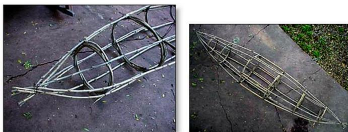
Completed frame. Length is 11.5'. Stringers are about 15' long and overlap the two center ribs. The center ribs are 27" wide and 16" deep. The next out from the center ribs are 19" by 14". The smallest ribs are 13" circles. Spacing of the ribs is 17", 17", 24", 24", 17", 17".
