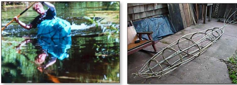
The amount of willow used to make the kayak. If you plan to build this kayak consider building a model. Making a model first of thin willow will make it easier to build a full size kayak. Waxed cord grips the willow and speed along the process. How about a two person boat?
