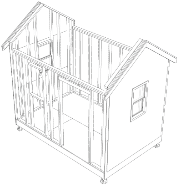
fig.12- Shed Framing Assembly
