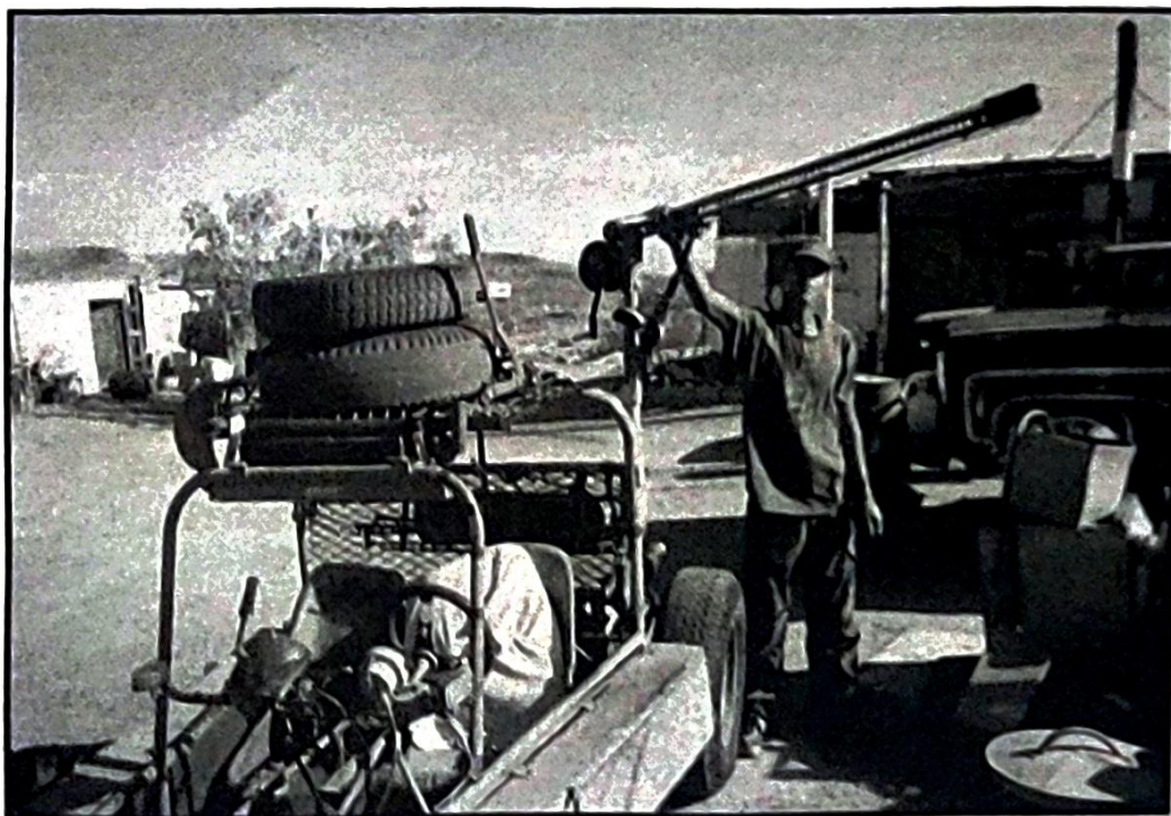
Boy Tuke with one of his homemade buggies. The hoist allows him, if necessary, to pull the engine and transmission in the field.
