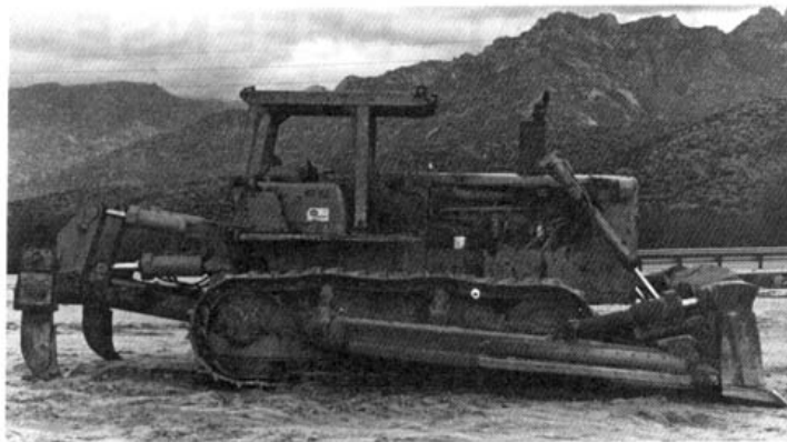
Bulldozer. Note the smoke stack (exhaust pipe).
