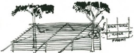
Cutaway section of frame for hut sited between two saplings
