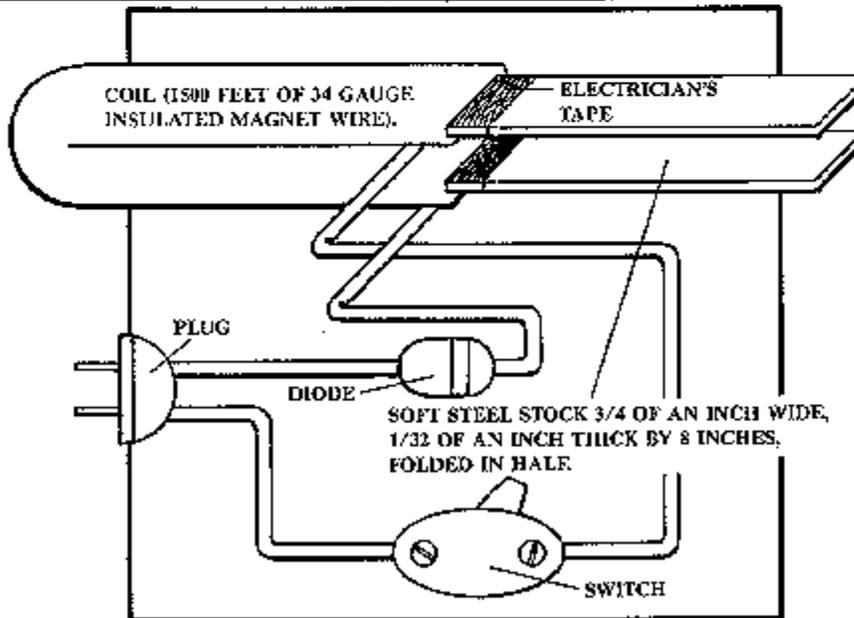
Figure 30. The magnetic pick is easy to construct.
